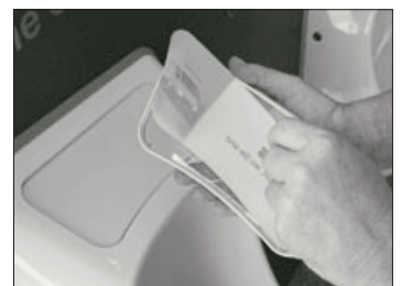
Insert Foil between plastic cover and external window...
